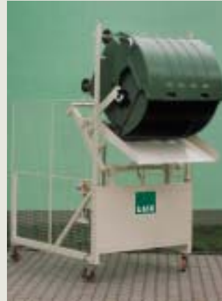
Easy emptying of container with compacted cardboard
