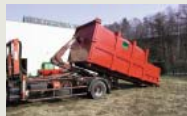
Loading of press container on collecting vehicle
