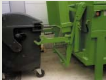
Detail of a built-in dumping equipment
