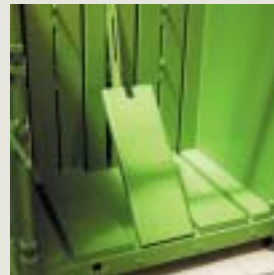
Hydraulic ejecting of pressed bale
