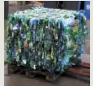
Pressed bale of PET bottles, 220 kg
