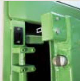
Encoded safety switch, in compliance with EN 60-947-5-1
