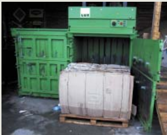
L30-2 - Double-chamber baler - example of ejecting a bale to a pallet - cardboard, 390 kg
