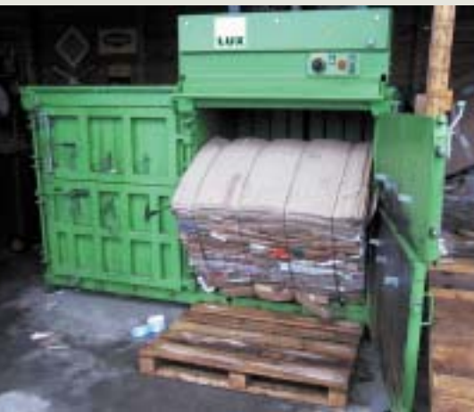
L30-2 - Double-chamber baler - example of ejecting a bale to a pallet - cardboard, 390 kg
