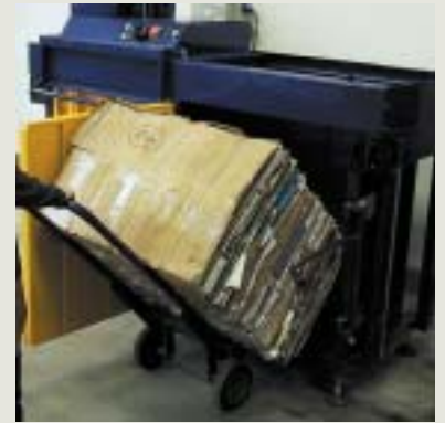
Easy removing finished bale from baler using a bale trolley
