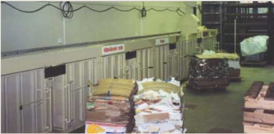
Ten-chamber baler configuration in AVX Lanškroun
