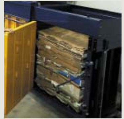
Pressed and strapped cardboard bale in the baler - bale weight 85 kg
